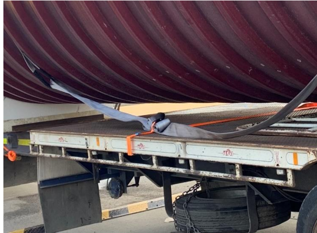
Picture 2 – Loose ends of slings secured to the deck of trailer
