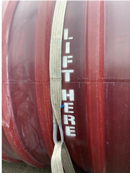
Picture 1 – Ensure sling is located over Flat marked 'Lift Here'
